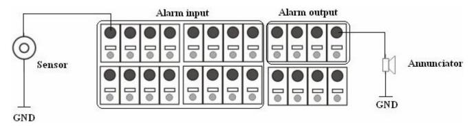
Attention: The alarm output is TTL high level control. The connection method is described in detail in the Above picture.
